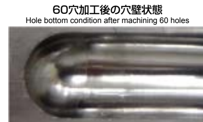
穴壁面粗さ Rz1.8μm Hole wall surface roughness Rz: 1.8 μm
